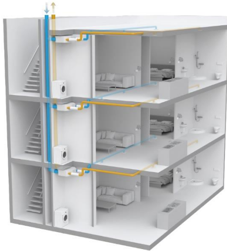
Overview ventilation system HRC-OptiAir EU
